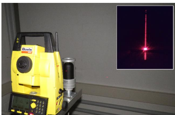
Figure 1 – Alignment between theodolite (point-laser) and Geovane (line-Laser)
