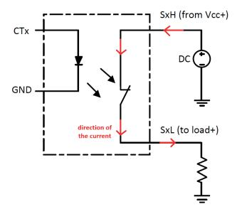
Please note the direction of the current: the current **must** enter through the H terminals and exit through the L terminals.
