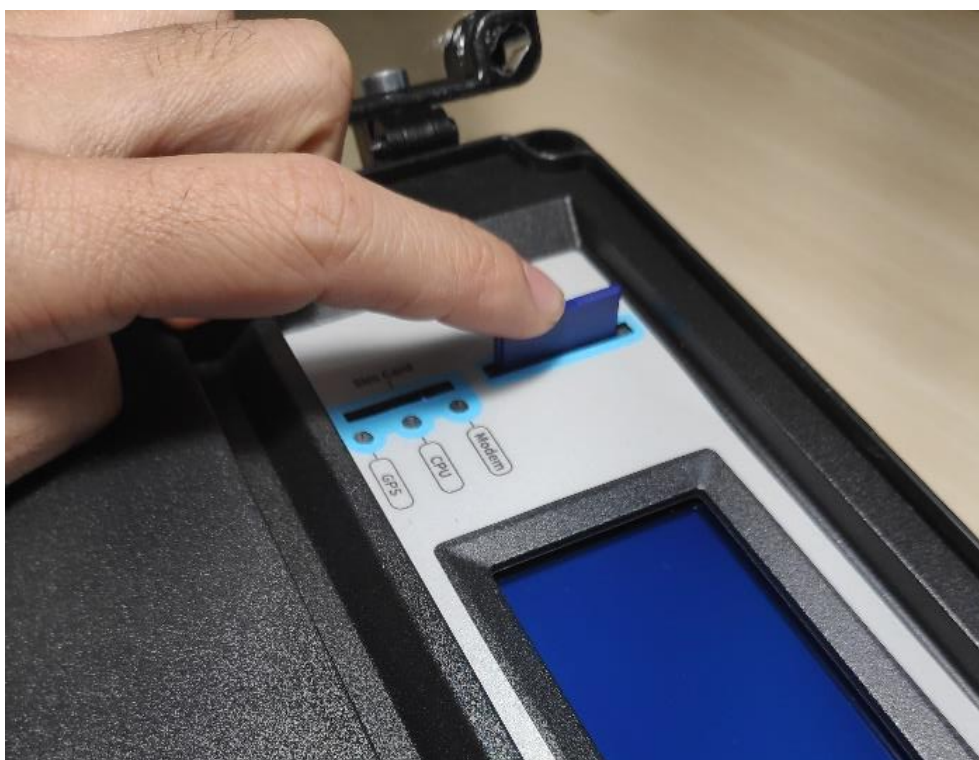
Fig. 56. How to take out the SD card
