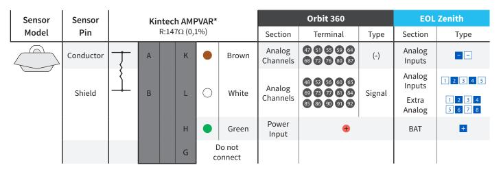
**Note:** \*AMPVAR amplifier is provided by Kintech Engineering. Consult to the Solar department (solar@kintech-engineering.com) for its configuration and Slope and Offset.
