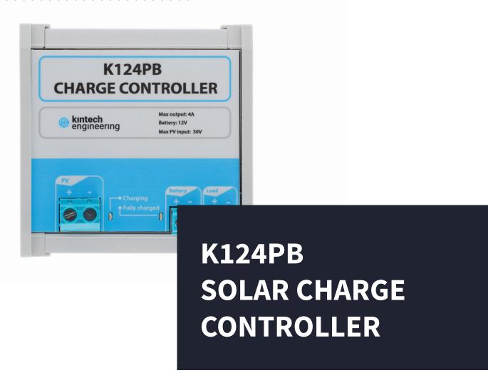
The K124PB serves as a battery charge controller with a special focus on maximizing battery lifespan and charging efficiency. It can be powered either by a solar panel or a DC regulated power supply. When connected to a solar panel, the regulator employs a Maximum Power Point Tracking (MPPT) algorithm, ensuring optimal system efficiency and maximum power output. The two LEDs on the regulator show the charging progress and indicate when the battery is fully charged.
