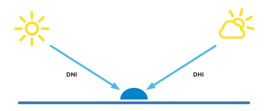
Global Horizontal Irradiation (GHI) = DHI + DNI x cos ( $\Theta$ )  $\Theta$  is the solar zenith angle
