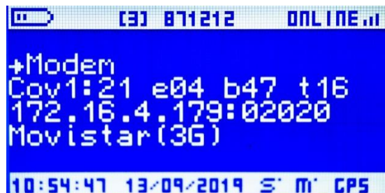
Fig. 70. Logger display: status > modem > e04 (logger online)
