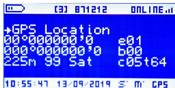
Fig. 37. STATUS screen: Site Coordinates
